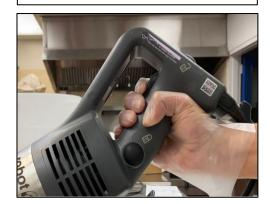
**Step 6:** Release the *safety button* while still holding the *control button* on the *main handle*.
