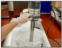
**Step 3:** Insert *tube* into container with the *bell* completely immersed and the *splash guard* in place.
