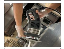
**Step 8:** To stop the power mixer, release the *control button* while holding the *removable handle*.
