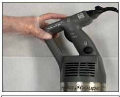
**Step 4**: Keep *safety button* pressed while completing Step 5.
