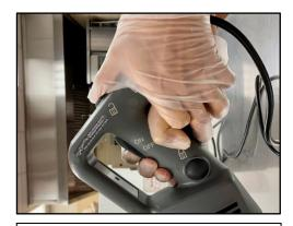
**Step 5:** Press and hold the *control* button on the main handle and the mixer will start.
